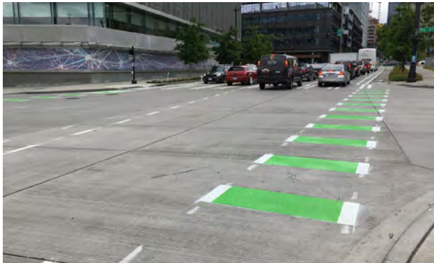
Bike lanes should continue through intersections
